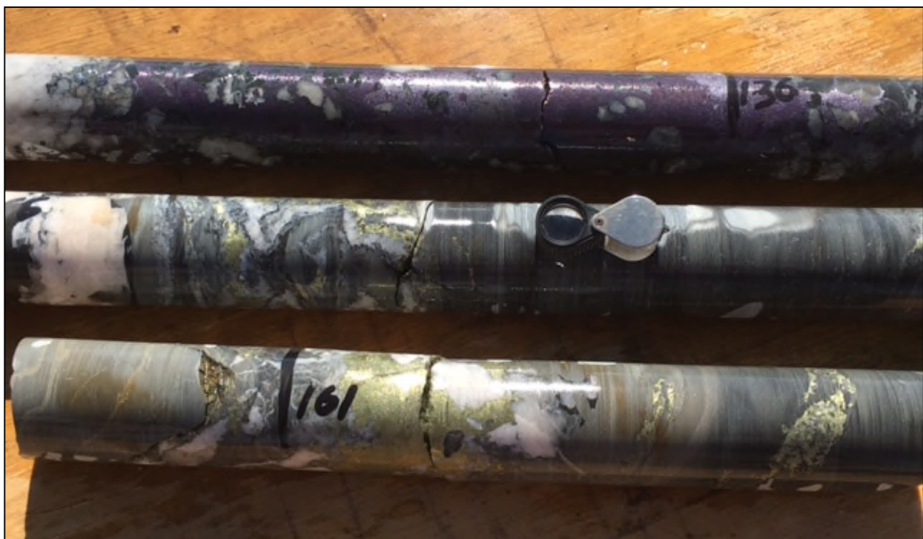
Figure 7: Vein hosted copper sulphides: bornite (top) and chalcopyrite (centre & bottom) in drill core from MO-G-16D
