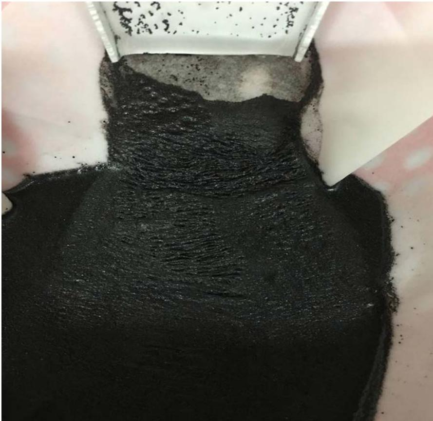
Figure 1: Agglomerated graphene produced from cell overflow
