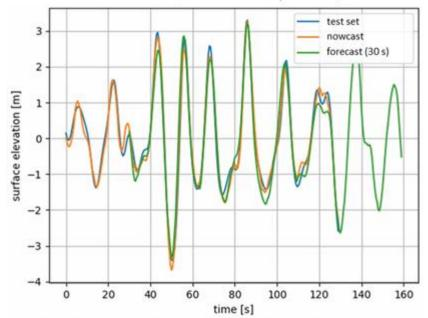
Carnegie's wave predictor results showing close correlation of the surface height elevation prediction 30 seconds ahead ('forecast (30 s)') to the actual data ('test set')
