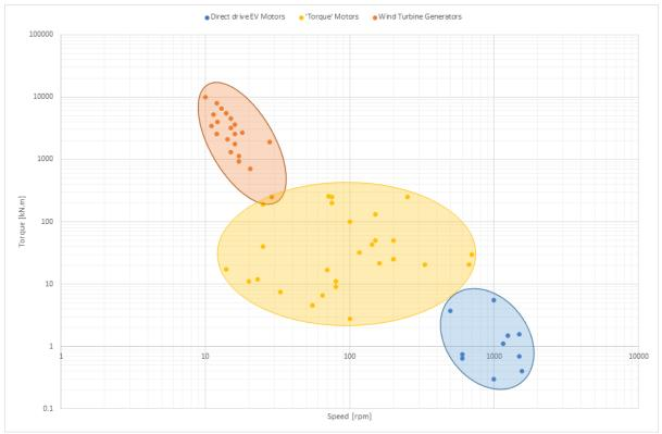
Nominal torque vs nominal speed for 59 different electrical machines investigated for use in the CETO device across a wide range of scales
