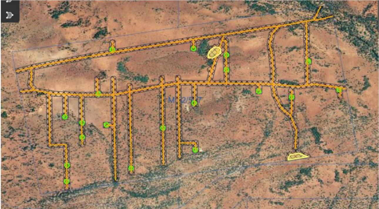
Figure 8. Location of the planned RC holes and access tracks.
