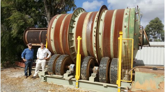
This trommel is the same one that was originally used at the Blina Diamond Project by the previous operators in 2005 and 2006. This equipment has been shown to be highly effective and fit for purpose for treating the alluvial gravel types which are encountered at Blina.
