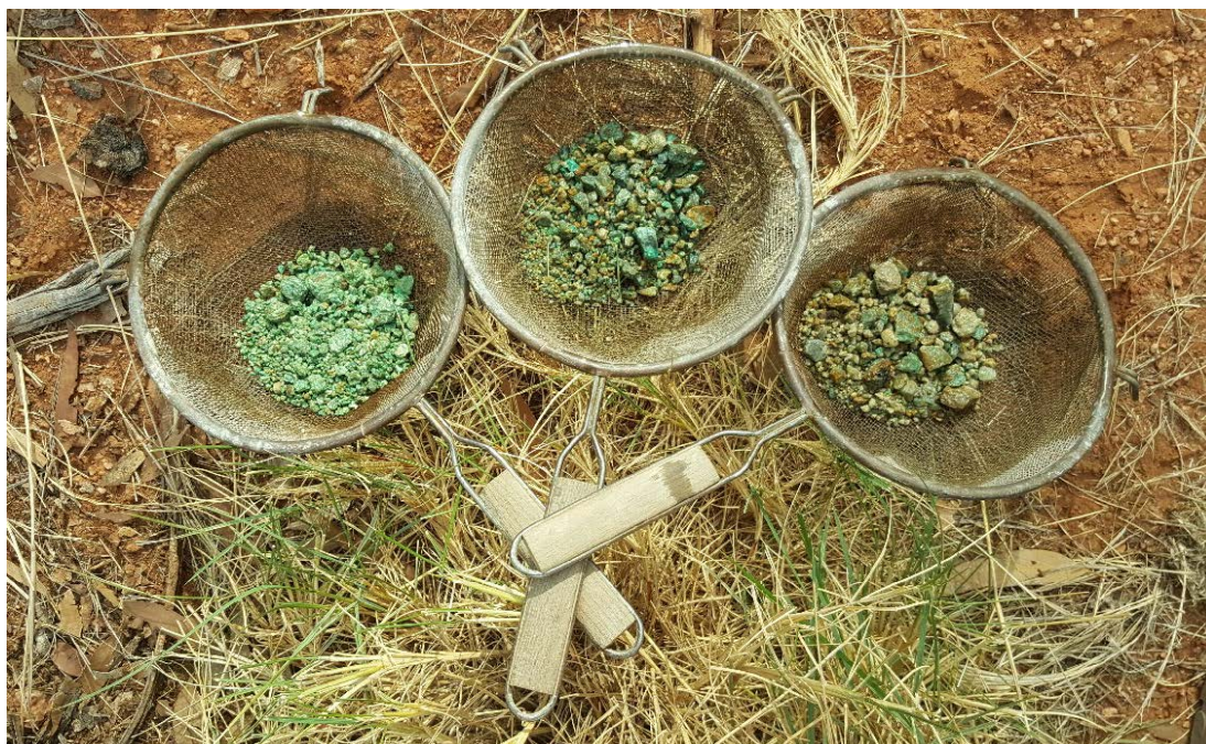
Figure 1: Copper oxide mineralisation (malachite) from drill hole CPR628 at Companion. From left to right; 5-6 metres 2.83% copper, 1.73g/t gold; 6-7 metres 2.96% copper, 0.65g/t gold; 7-8 metres 2.28% copper, 1.81g/t gold.
