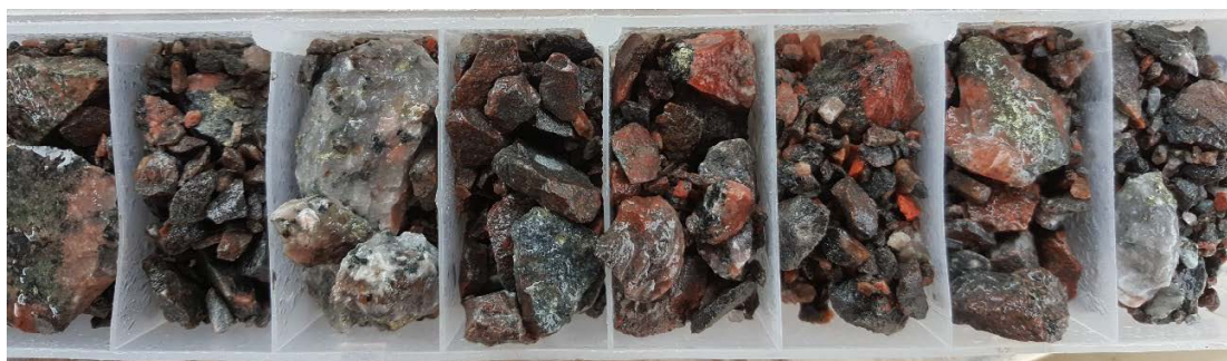
Figure 2: Red rock alteration and chalcopyrite mineralisation typical of IOCG deposits from 51-55 metres in CPR633 from Companion. Copper grades range up to 0.78% with gold up to 0.44g/t.
