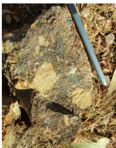
Figure 3: Copper mineralisation (malachite and chalcocite) within outcropping breccias typical of IOCG deposits from historic workings at the Veiled prospect.
