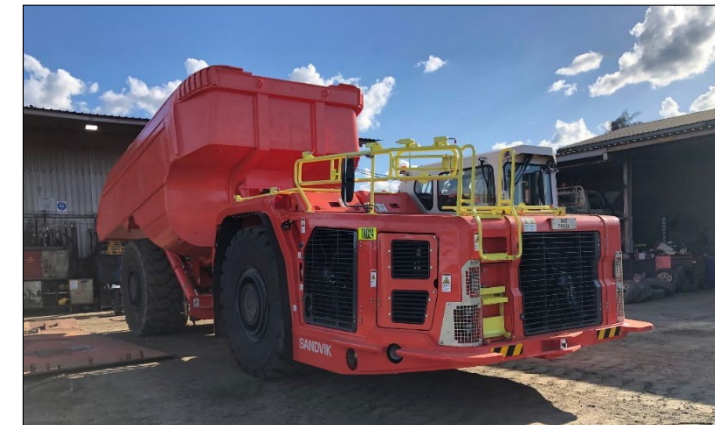
Truck 24 (Sandvik TH663) after a mid-life rebuild February 2023
