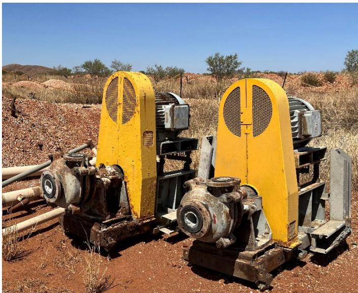
**Figure 8** - Removed and successfully rebuilt process water pumps
