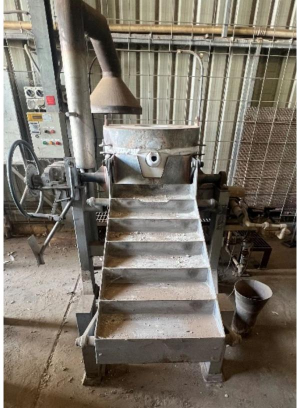
**Figure 4 –** Furnace replaced complete with new spout & crucible
