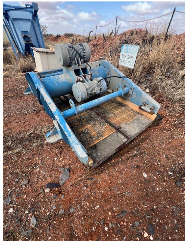
**Figure 7** – Tailing Screen removed to replace the underpan
