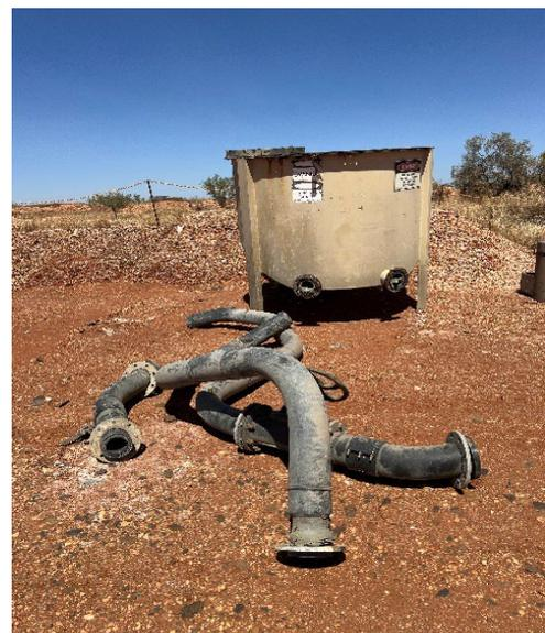
**Figure 9** – Removed pre-leach thickener hopper to be re-lined
