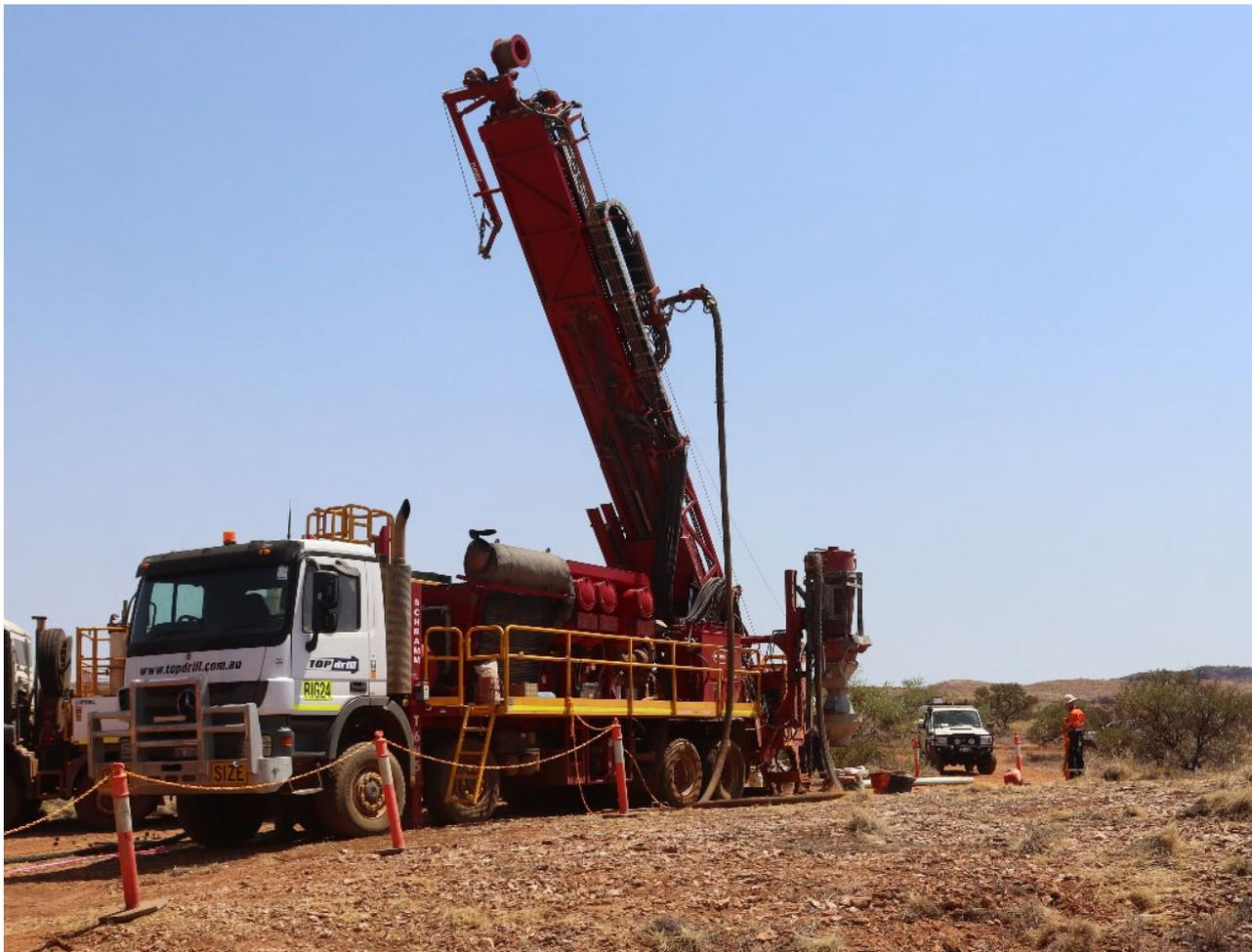
Figure 3: Topdrill Rig 24 RC drilling at Paulsens East in November 2023.
