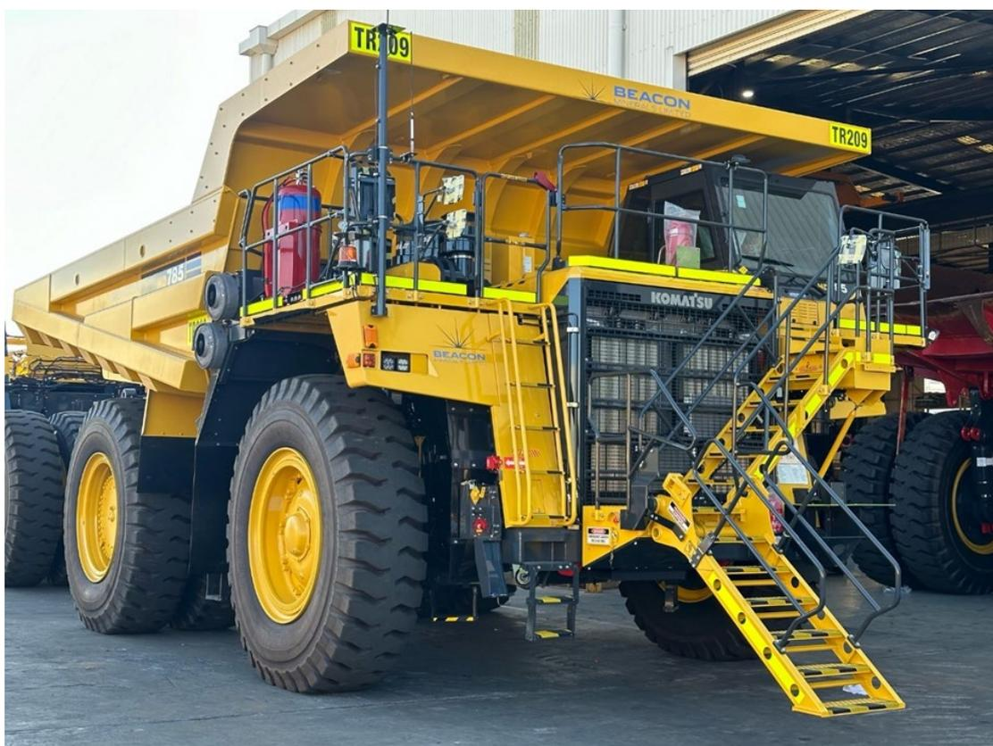
Figure 3 - New Komatsu 785-7 (92 tonne) truck ready for despatch from Welshpool
