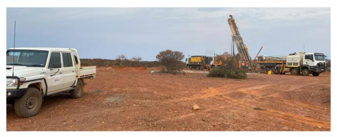
Figure 1. Orlando Drilling reverse circulation rig commencing drilling at the Southern Star prospect.
