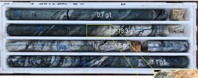
Figure A. Diamond core from SDD015 from 105.95m to 109.59m with visible gold at 107.4m in HQ (63mm diameter). SDD0015 intersected a quartz-rich laminated shear vein from 107.3m to 109.2m, within a broad 28m wide zone of extensional quartz veins, with distinct haloes of coarse-grained pyrite, from 88.5m to 116.5m, Overall intercept assayed 30m @ 3.0 g/t gold, incl. 1m @ 18.3 g/t gold from 107m
