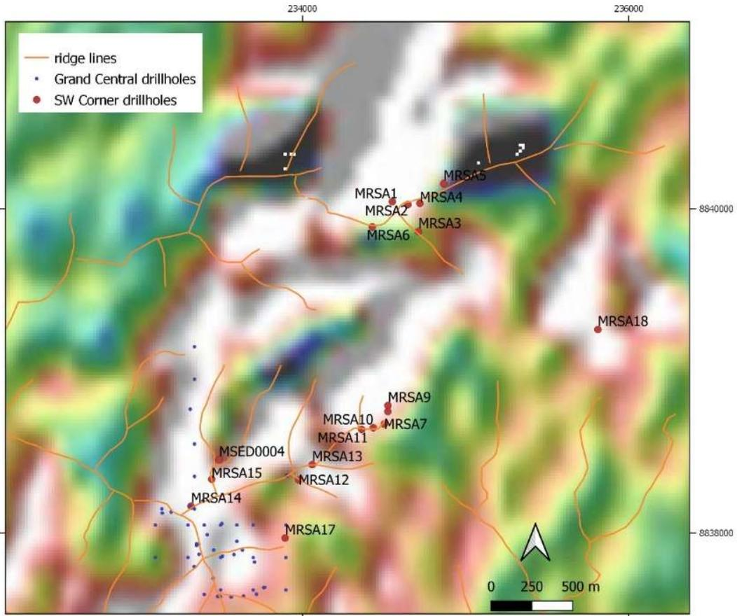
**Fig 4: SWC target area and airborne radiometric data with drill holes (white is highest radiometric intensity)**
