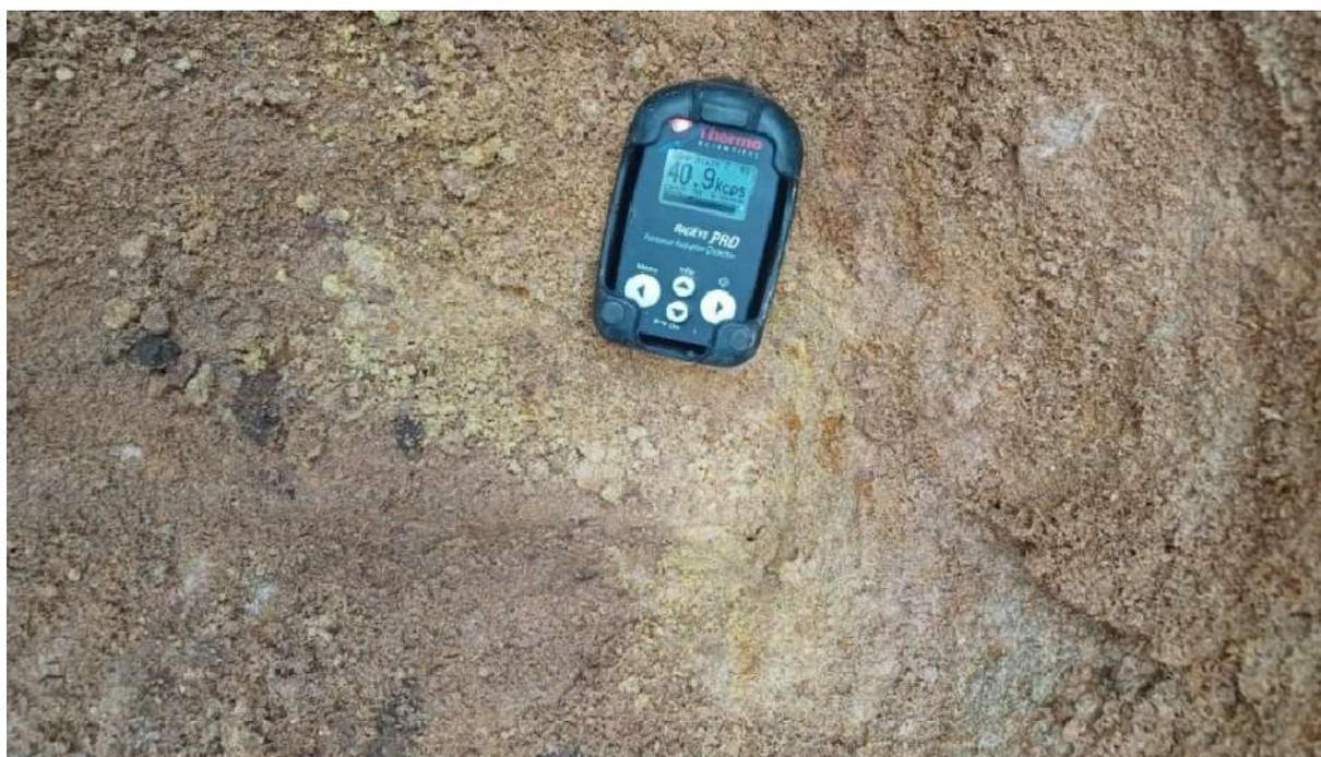
**Fig 3: High-grade Uranium mineralisation in saprolite at Mtonya-SWC trend (an extremely high 40,900 counts/sec)**
