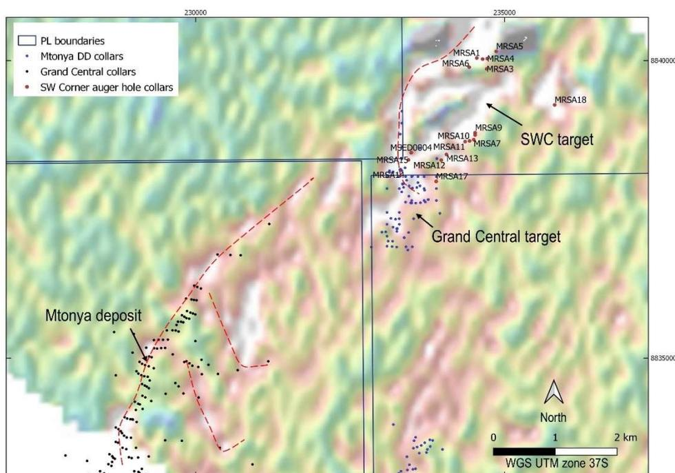
**Fig 2: Airborne radiometric data (highest intensity in white) over the Mtonya-SWC trend, with SWC & historic drill holes**
