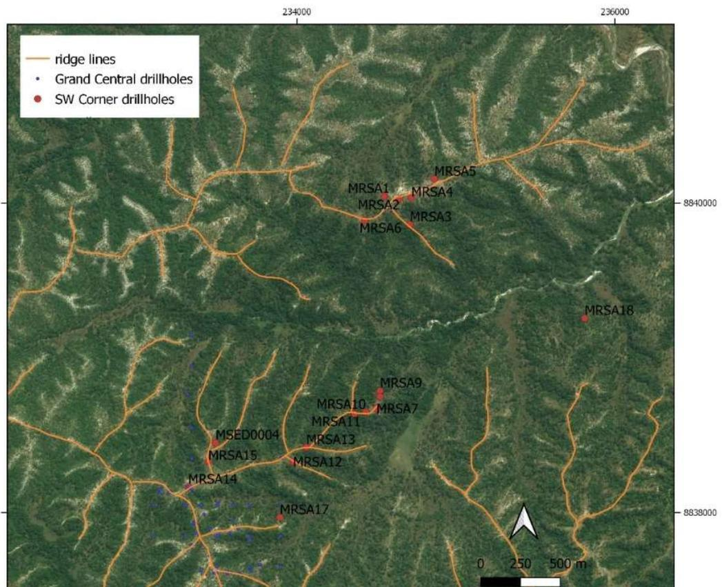
**Fig 5: Same area as Fig 4 on satellite background. All holes drilled on ridge lines (orange lines) with valleys between**
