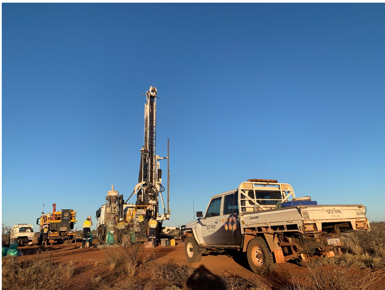
Photo 1. Strike Drilling T450 Aircore/Reverse Circulation Rig
