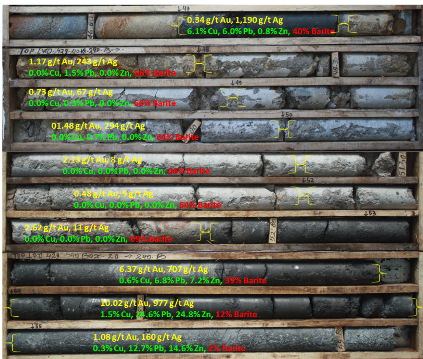
Figure 1: Photograph of diamond drill core from hole LWD 429. The photo was taken prior to sampling. Please note the association of very high base metal and silver assays with the darker, sulphide-rich “black smoker” mineralisation. The pale barite-rich “white smoker” style is low in base metals but carries elevated gold values.
