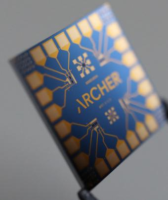
Lab-on-a-chip device integrating graphene biosensors with the potential to parallelise the detection of biologically relevant targets.
