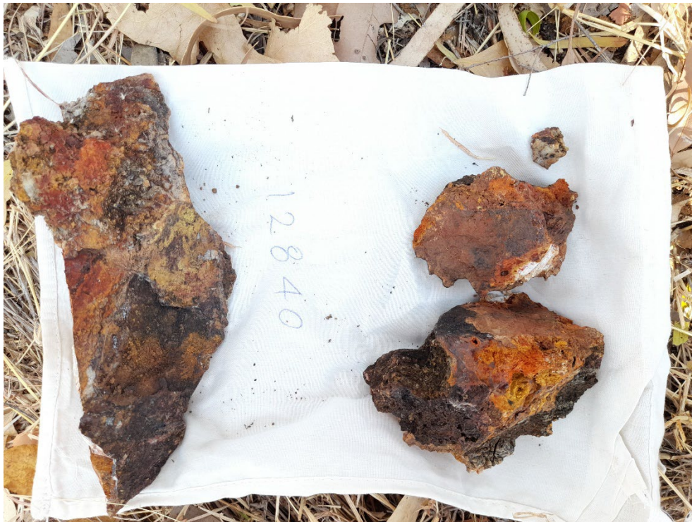
PLATE 2: Sample 12840, of mullock from shallow pit west of the main Pinnacles workings, composed of vughy quartz vein material with limonite boxworks after sulphides (11.95 g/t gold).
