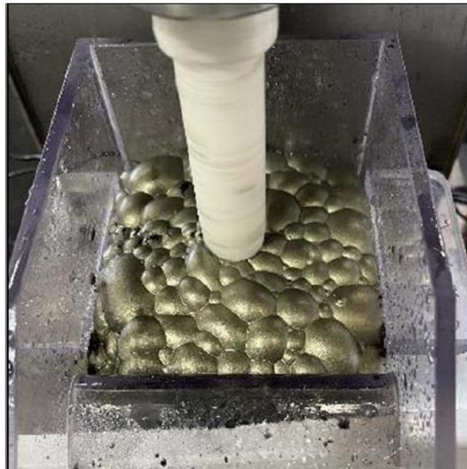
*Figure 20. Image of cleaner concentrate from Lady Colleen metallurgical testwork*
