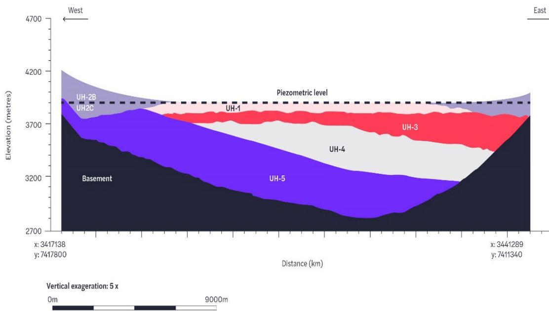
**Figure 4: Geological model of the Olaroz salar looking north through the northern part of the basin**
