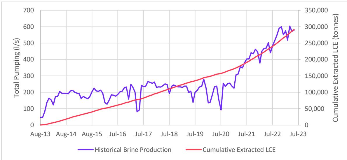
**Figure 2: Production Wellfield Pumping and Extracted Lithium in Brine to ponds (August 2013 to June 2023)**
