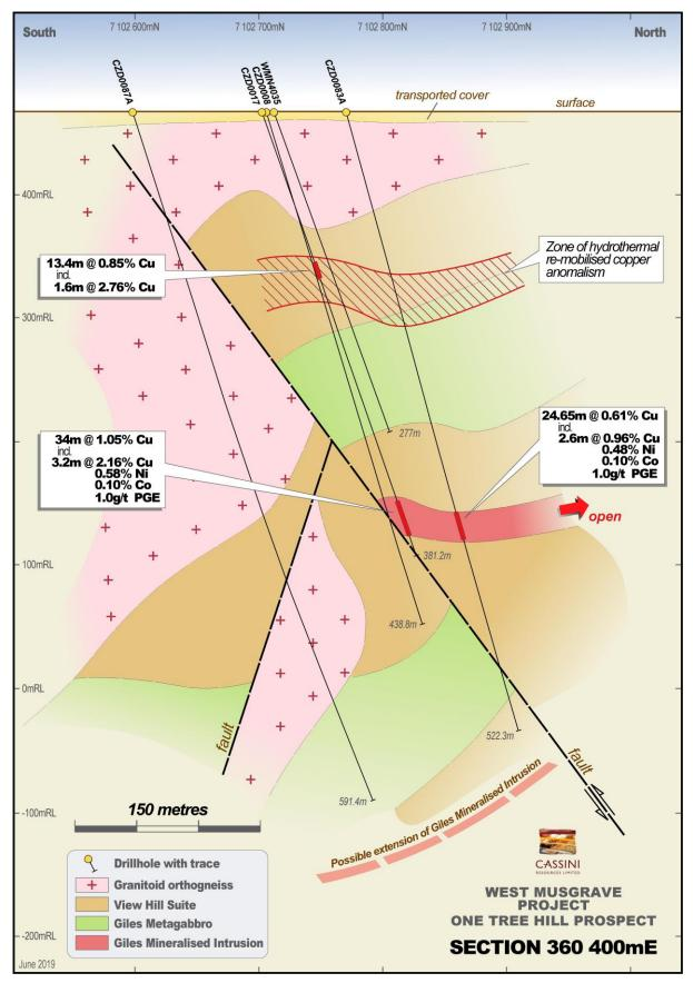
**Figure 4**. Section 360400E showing results of previous drill programs. The upper zone of hydrothermal copper mineralisation and anomalism is considered to correlate with Zone A in CZD0099.
