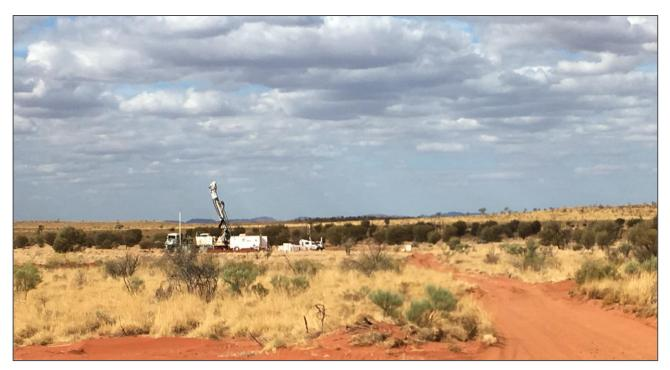
Figure 3. Diamond drilling operations at One Tree Hill. Note the extensive sand cover, including sand dunes in the background, which obscures bedrock.
