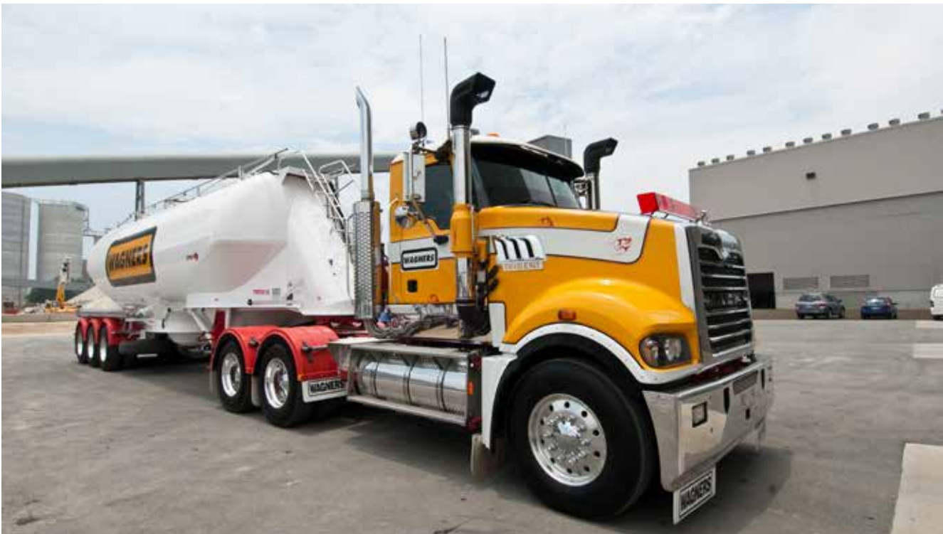
FIGURE 25 Wagners’ pneumatic cement delivery equipment
