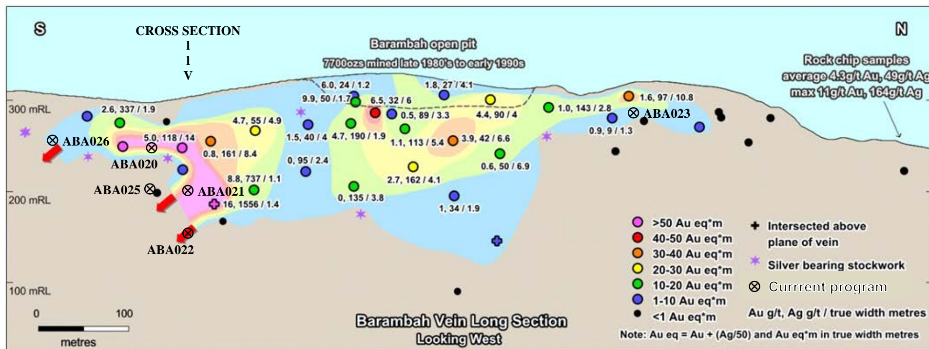
Figure 2: Barambah vein – Long Section showing current and previous drill holes, old mining area, and south plunging high grade shoot interpreted from previous drilling information (previous holes and coloured contours colour coded in gold equivalent gram-metres – not updated with current drill information – see JORC Section 2 for explanation of aggregation method)
