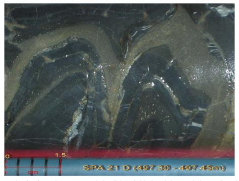
Pyrite lamina and veins in carbonaceous shale, tightly folded and dragged along micro faults which are partially occupied by quartz-carbonate veins. This type of structure is also observed at Anjing Hitam and Lae Jehe.
