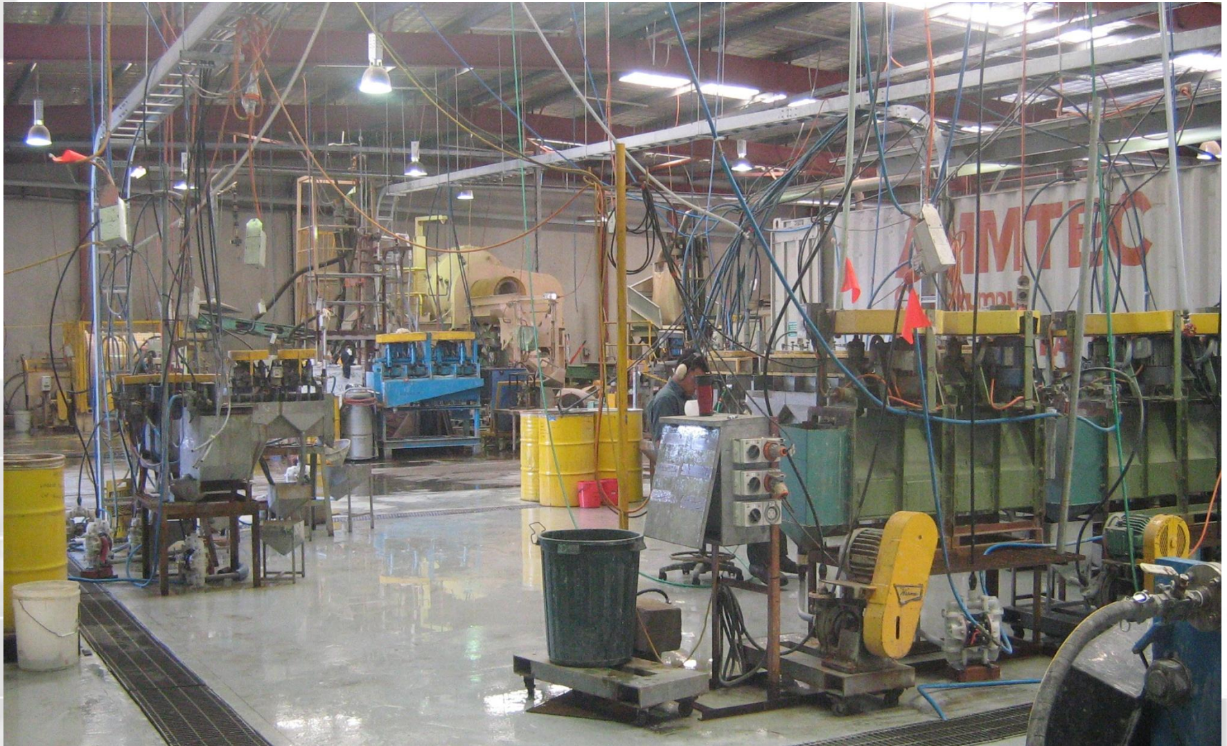
Pilot Scale Flotation Plant, set up to duplicate on site plant at a rate of 500Kg/hr
