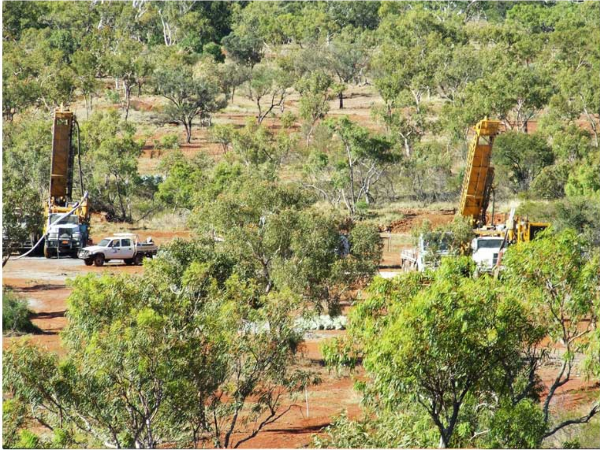
Two large RC Drill Rigs drilling in tandem at the S.E. end of Las Minerale further extending the strike length of Las Minerale
