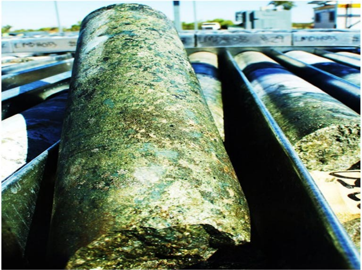
Section of wide diameter PQ Diamond drill core in 7 m drill tray showing core impregnated with massive sulphides containing chalcopyrite and chalcocite (high grade copper mineral)
