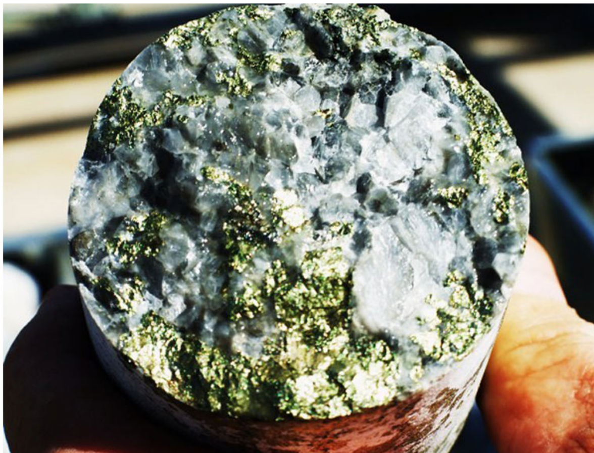
Diamond core with heavy duty chalcopyrite in calcite and quartz rock.
