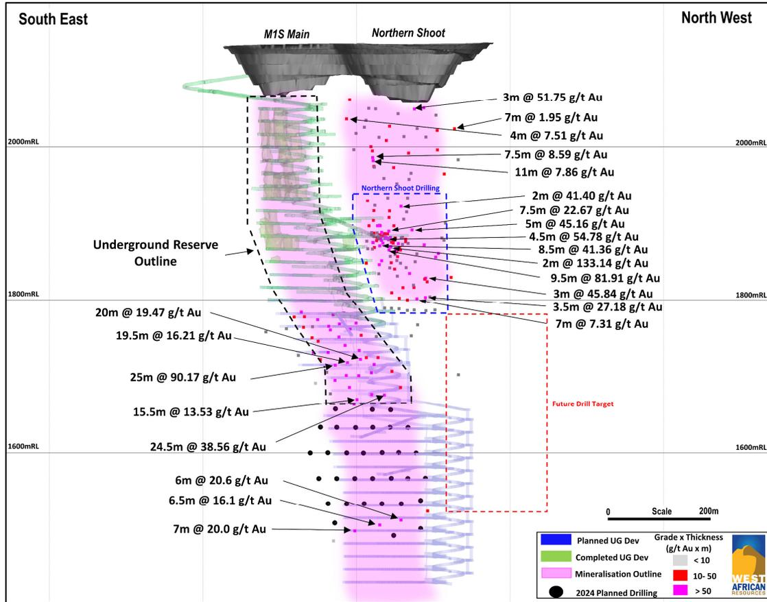
Figure 3: Long Section of M1S Northern Shoot Drilling
