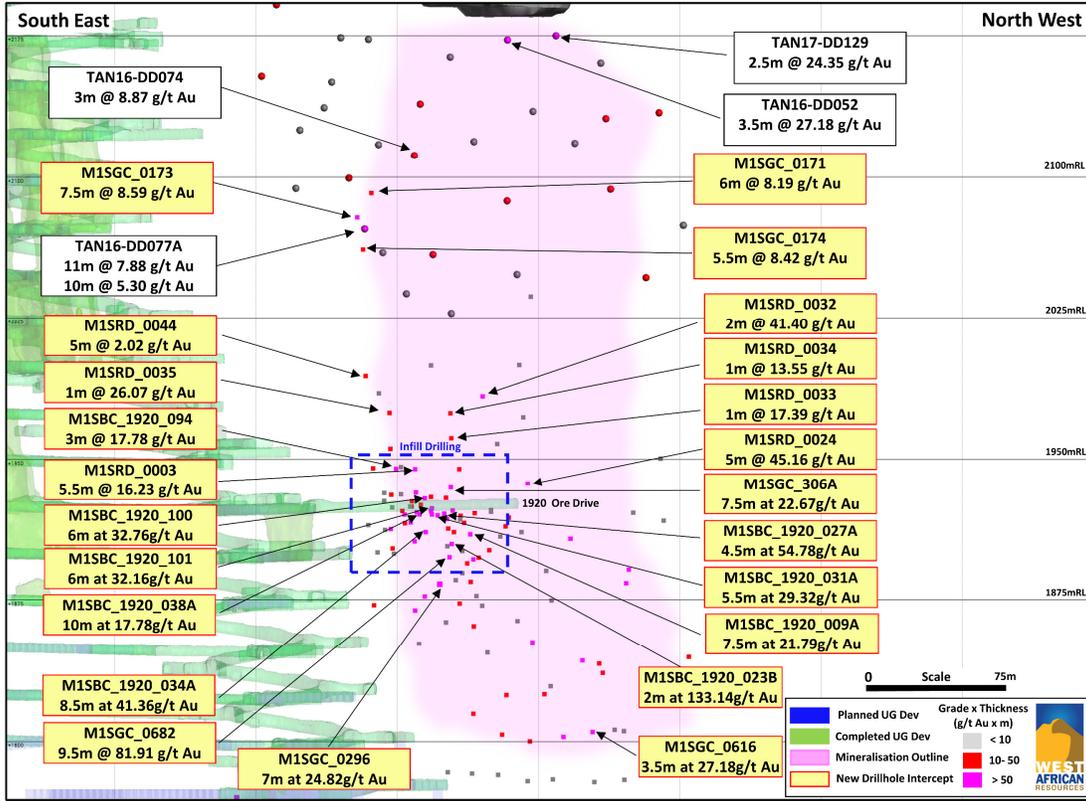
Figure 4: Oblique view of the M1S Open Pit Northern Shoot Model
