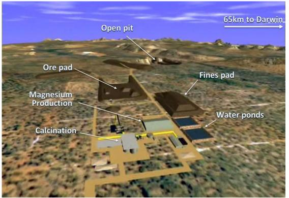
Figure 9 Layout of the Winchester magnesium plant and mine based on the technology using electric arc furnace and magnesium oxide, aluminium and ferrosilicon as feedstock.
