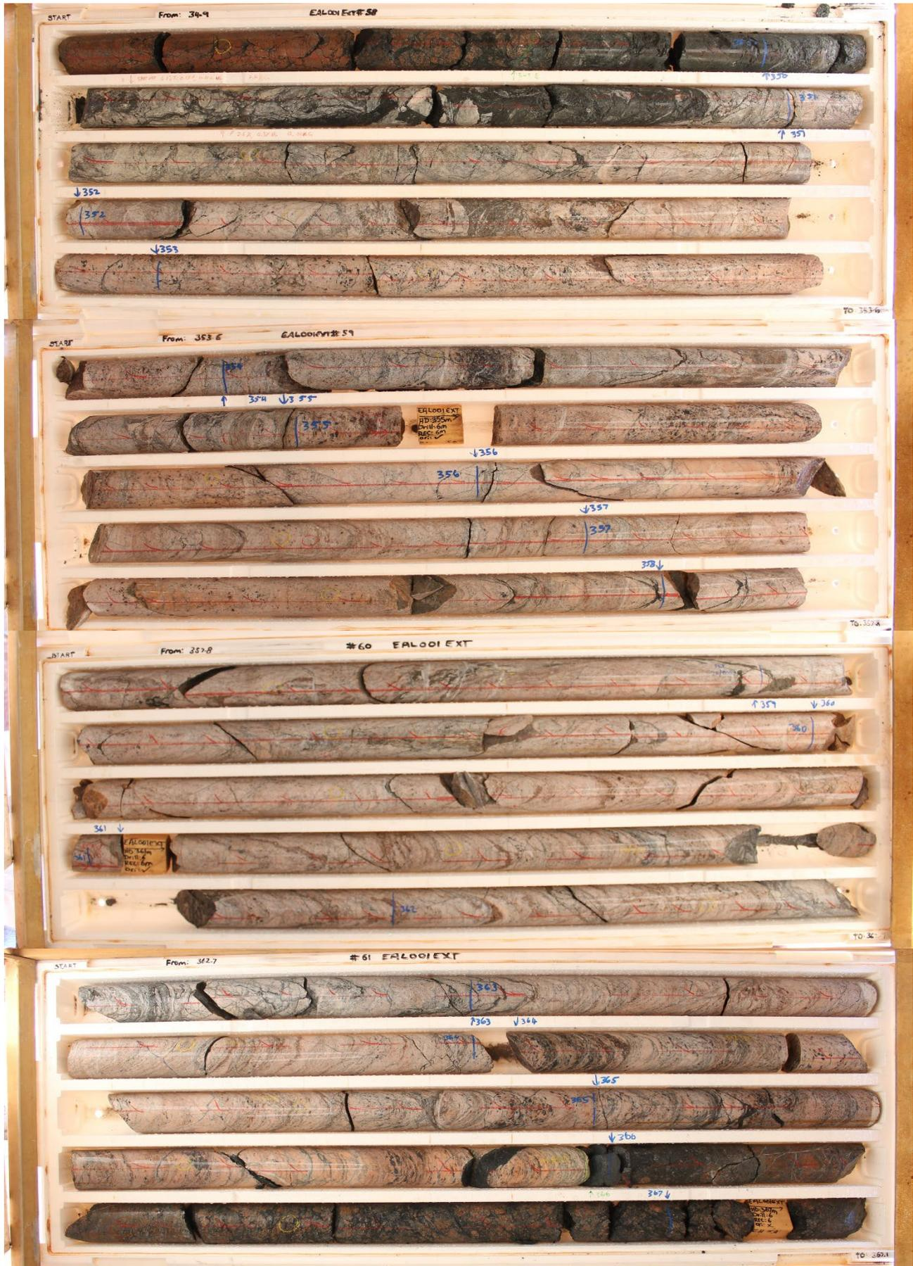
Photo 2 – EAL001 – Core photos 349-367.1m containing mineralised carbonatite intersection of 16m at 0.6% N<sub>2</sub>O<sub>5</sub> & 0.2% TREO (including 402ppm Nd+Pr) from 350m.
