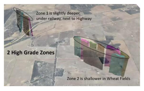
The CSIRO Magnetite Model (Burracoppin deposit). Modelled magnetic bodies are shown superimposed on the satellite image. The figure shows the separation of the magnetite mineralization into two higher grade zones.
