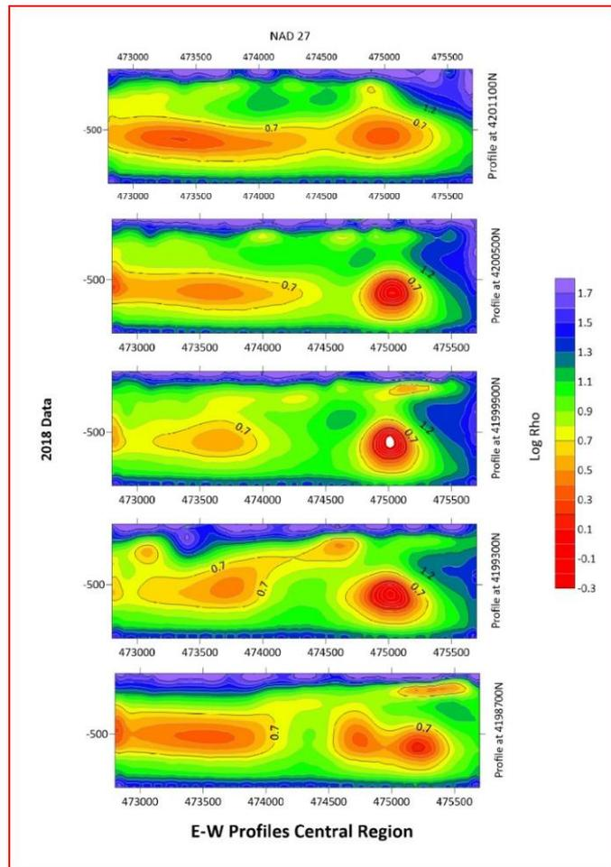
Figure 4. Stacked east-west profiles showing resistivity contours (5 ohm-m has a log value of 0.69 and resistivities are as low as 0.5 ohm-m which is a log value of -0.3)
