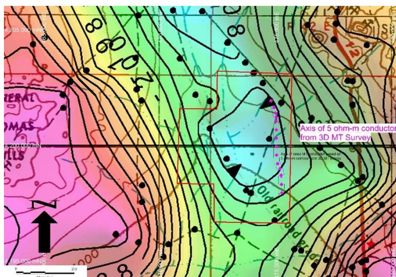
*The position of the tubular target (5 ohm-m conductor) is shown on regional gravity contour image where the Alkali Lake North Project area (outlined within red boundary) covers a gravity low. The tubular conductor is represented by mauve diamonds forming a line near the eastern boundary of the Project area.*
