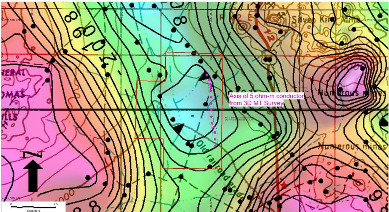
Figure 5. Gravity image for Alkali Lake Basin showing RLC claim block (red outline) and axis of 4.3 km long, 5 ohm-m conductor. NAD 27 Zone 11. Gravity image acquired from USGS PACE compilation.
