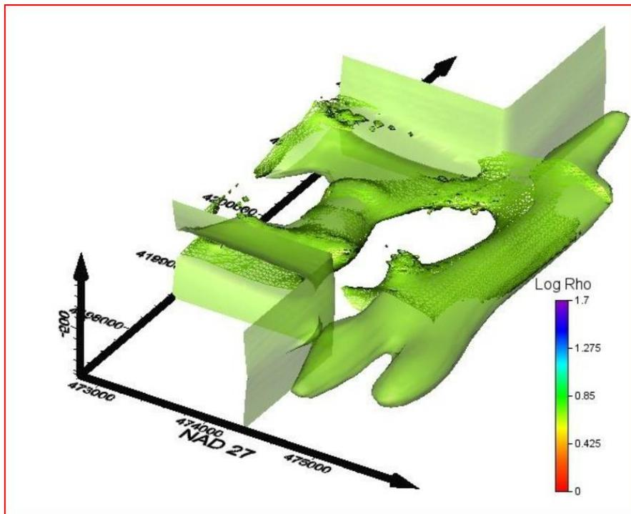
Figure 3. 5 ohm-m conductive shape outline viewed from south-east. Note that the Rho scale is logarithmic and 1 Rho is equivalent to 1 ohm-m, or 0 on the logarithmic scale; 5 ohm-m is 0.69 on the Log Rho scale.
