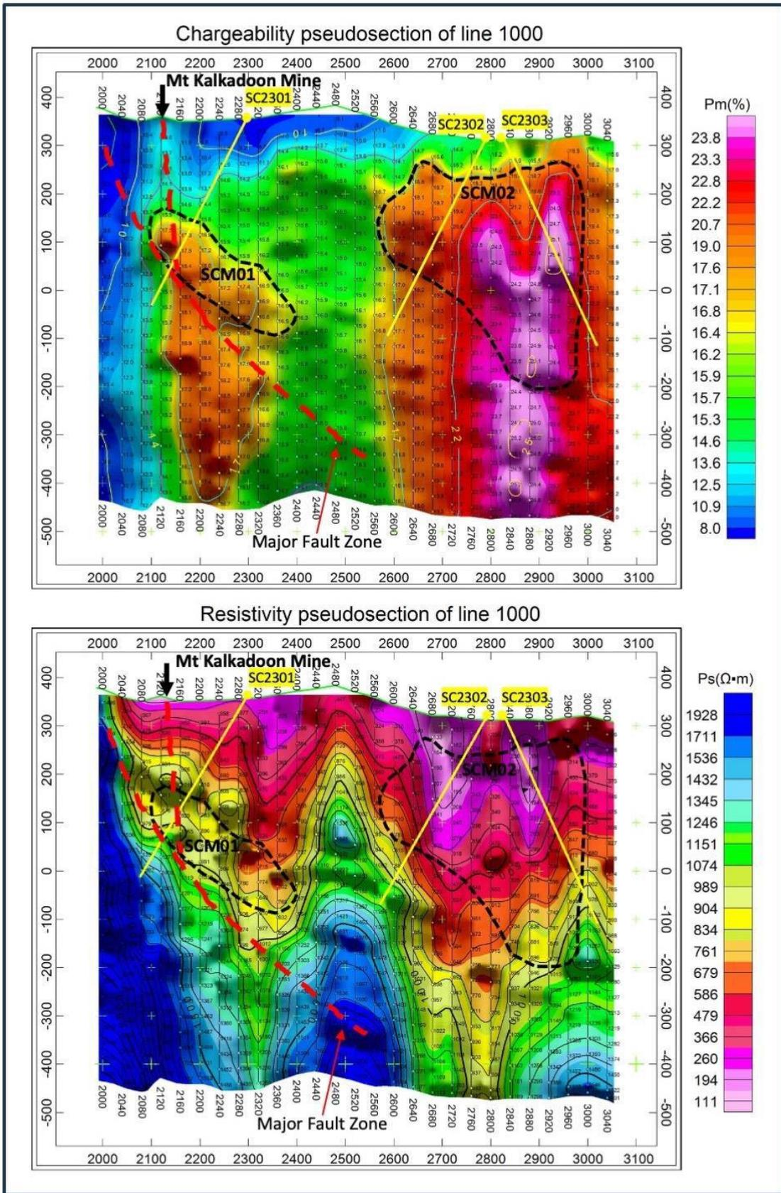
**Figure 5.** - 2D chargeability pseudosection (top) and resistivity pseudosection (bottom) of Line 1000 over the Mt Kalkadoon Mine. Note that SCM01 is about 250m below the known ore zone but sits above a major fault zone.
