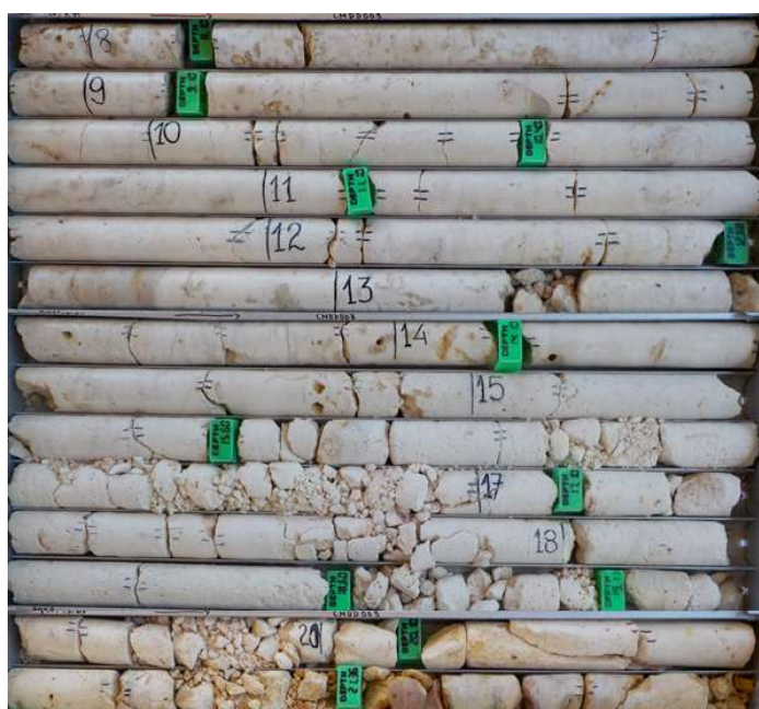
Fig 3 – “HIGH” purity core (CMDD003), 8.00 to 21.30m, weighted average 54.92% CaO (98.04% \text{CaCO}_3 Limestone)
