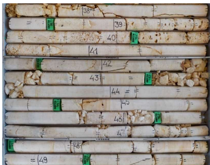
Fig 2 - VERY HIGH purity Limestone (CMDD008) from 37.88 to 49.53m, with weighted average 99.29% \text{CaCO}_3
