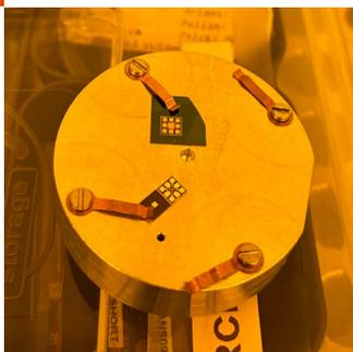
Archer’s biochip innovation aims to integrate graphene field effect transistors (“gFETs”) into advanced fluidic systems to create miniaturised lab-on-a-chip device platforms for medical diagnostics.
