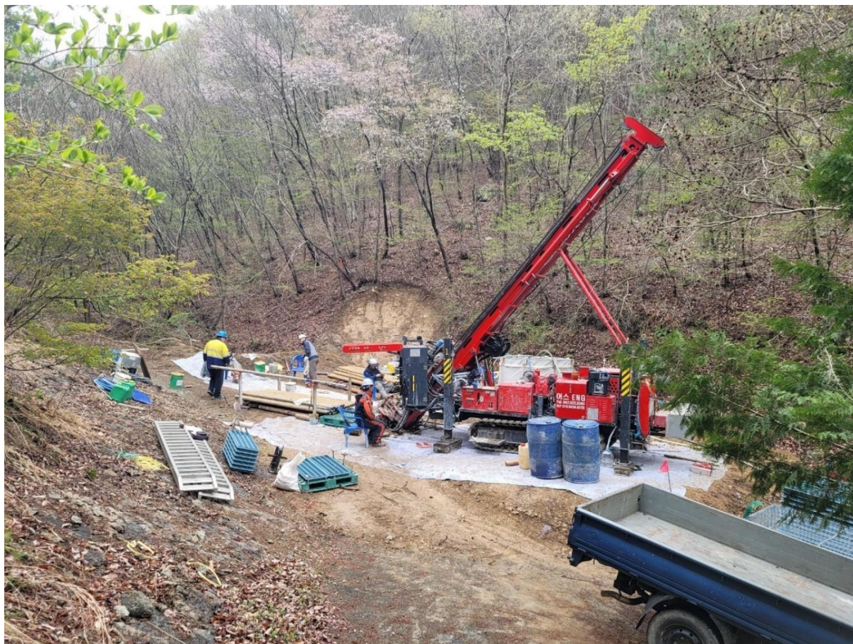
Figure 1: Diamond drilling of drillhole DKDD016 at Thorn-Nettle target at Deokon completed last week.
