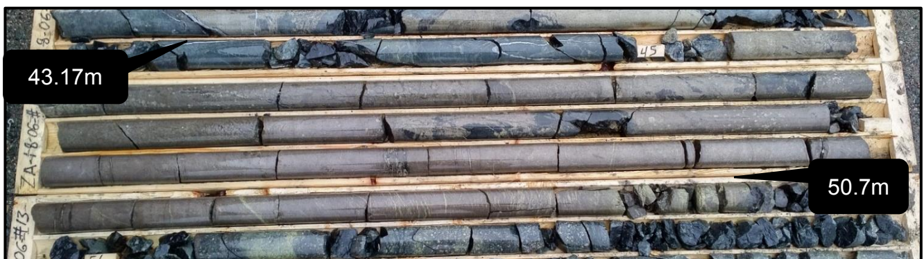
Figure 1: ZA-18-06 - Upper massive pyrrhotite-pyrite zone from 43.17 to 50.70m (7.53m)
