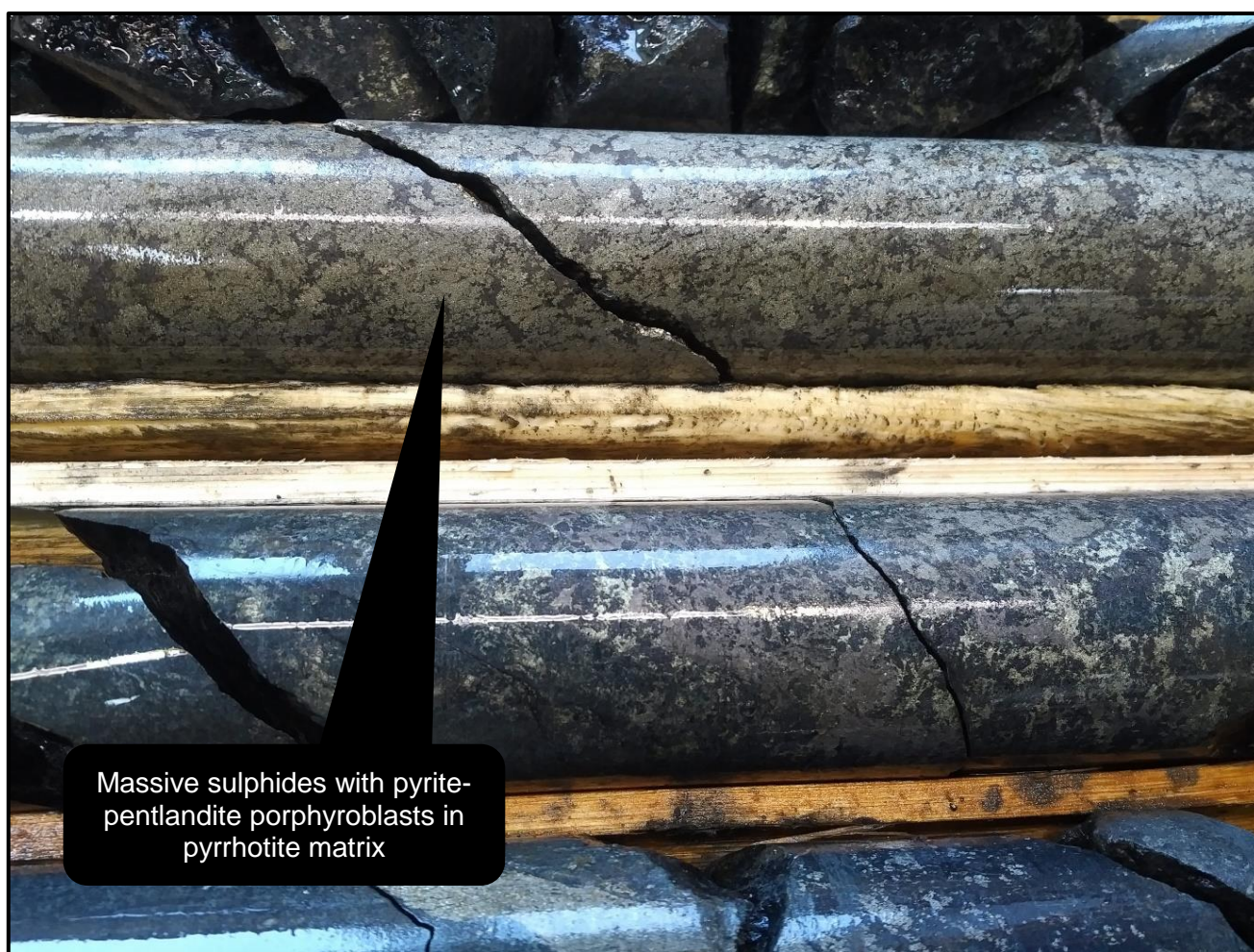
Figure 2: ZA-18-02 – Massive sulphide with coarse grained pyrite and pentlandite porphyroblasts in pyrrhotite matrix
