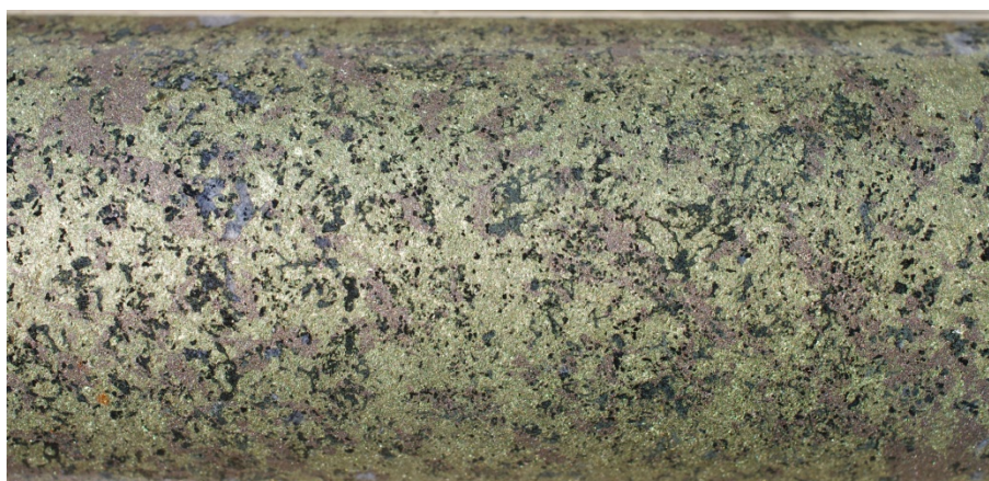
Figure 1: Close-up of massive sulphides intersected in diamond drill hole EMCDD056.
