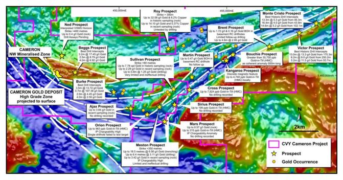
**Figure 3.** High-resolution Total Magnetic Intensity (TMI) image of some of the known gold deposits, prospects and occurrences associated with large-scale structures including the Cameron and Monte Cristo Shear Zones within the Company's Cameron Gold Project.
